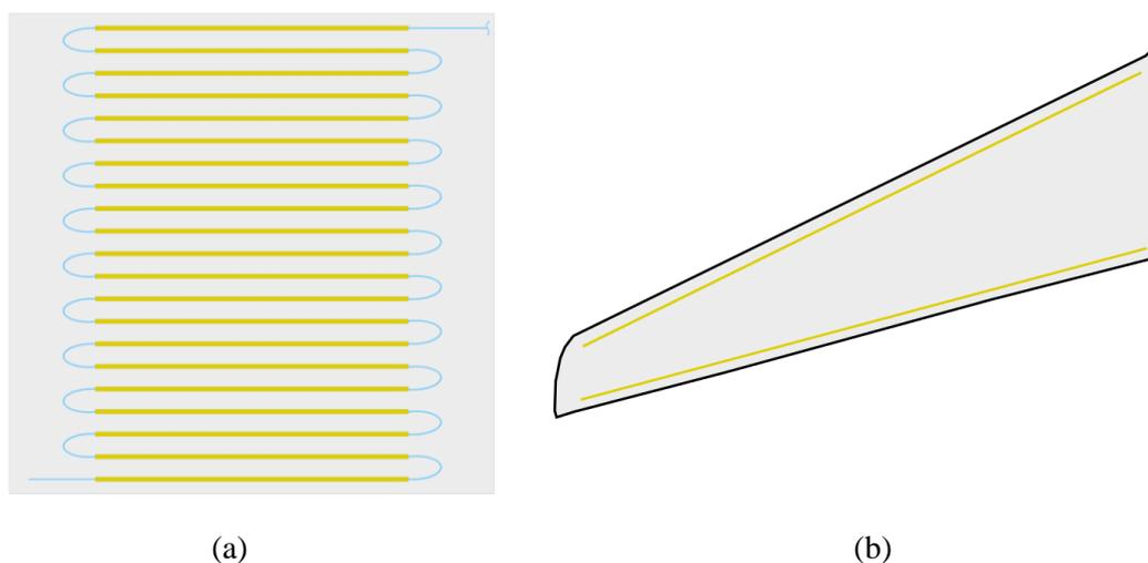
**Figure 2:** (a) The general installation strategy for complex layouts that require turns and bends. Only the straight segments of fiber are housed inside a tubing while the fiber bends remain free. If no turns or bends are required, the entire length of fiber may be packaged, as illustrated in (b).
