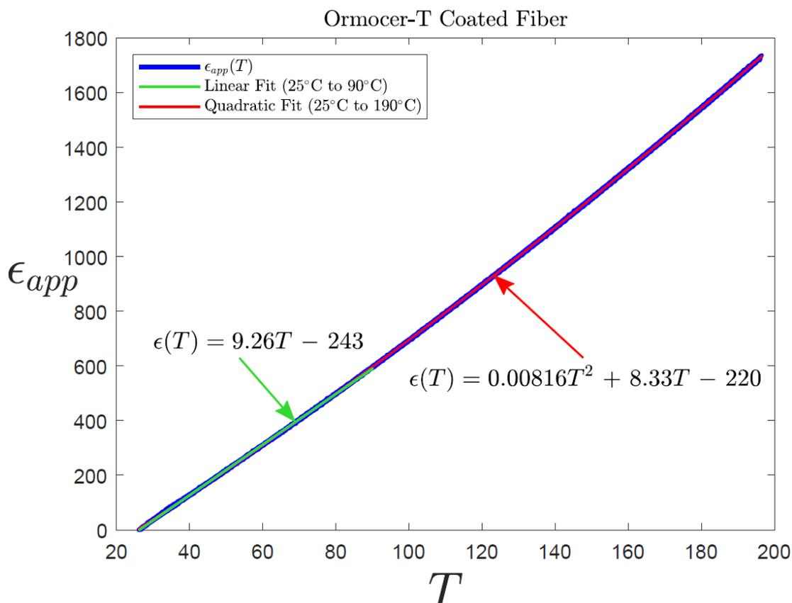
**Figure 4:** The temperature sensitivity of Ormocer-T coated fiber is shown. The sensitivity is effectively linear from 25°C to 90°C at approximately 9.2μ $\epsilon$ /°C. Beyond 90°C, a higher order polynomial calibration is required as the sensitivity becomes nonlinear.
