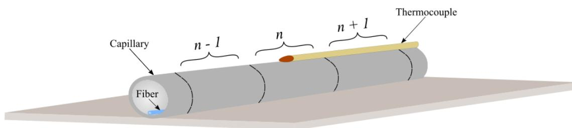
**Figure 3:** A thermocouple is positioned at fiber optic sensor  $n$  to monitor the local ambient temperature. The thermocouple data and measured apparent strain at sensor  $n$  are correlated to generate a polynomial calibration curve. For optimal calibrations, thermal paste or heat conductive tape should be used at the thermocouple interface.
