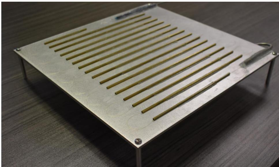
**Figure 6:** Several short segments of brass are utilized to achieve the desired spatial coverage. Depending on the chosen operational spatial resolution, the 2.5 m sensor length is comprised of between 100 and 1600 temperature sensors.
