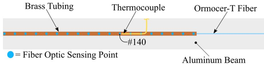
**Figure 7:** The corresponding fiber optic (FO) sensor number (#140) is identified and recorded. Thermal paste is used at the thermocouple interface to minimize the temperature difference between the thermocouple and fiber optic sensor.
