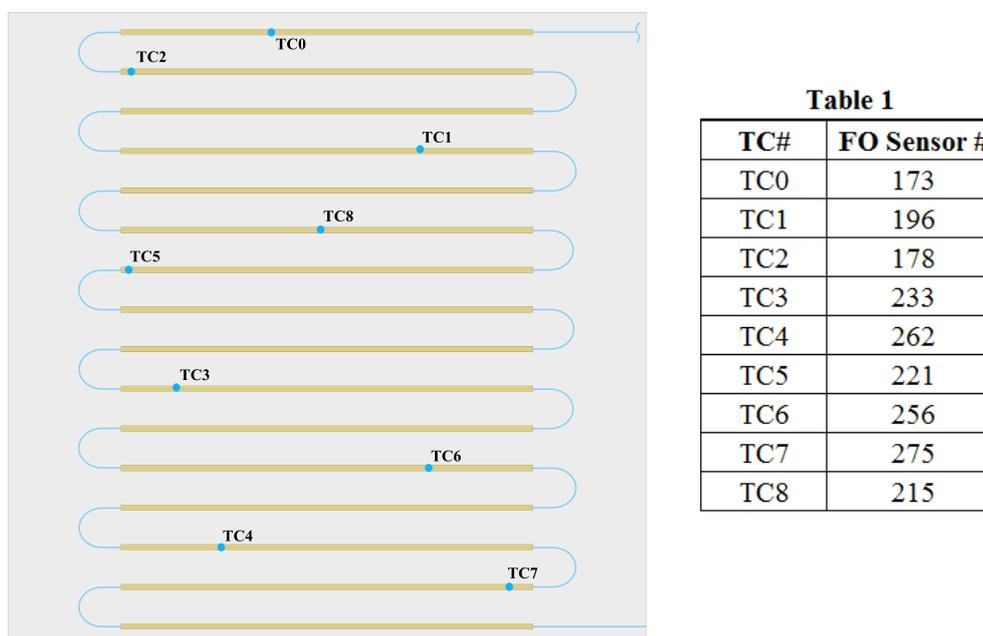
**Figure 9:** The locations of the 9 thermocouples are shown. At each thermocouple location, the corresponding fiber optic (FO) sensor number is identified and recorded in Table 1. Thermal paste is used at each thermocouple interface to minimize the temperature difference between the thermocouple and fiber optic sensor.
