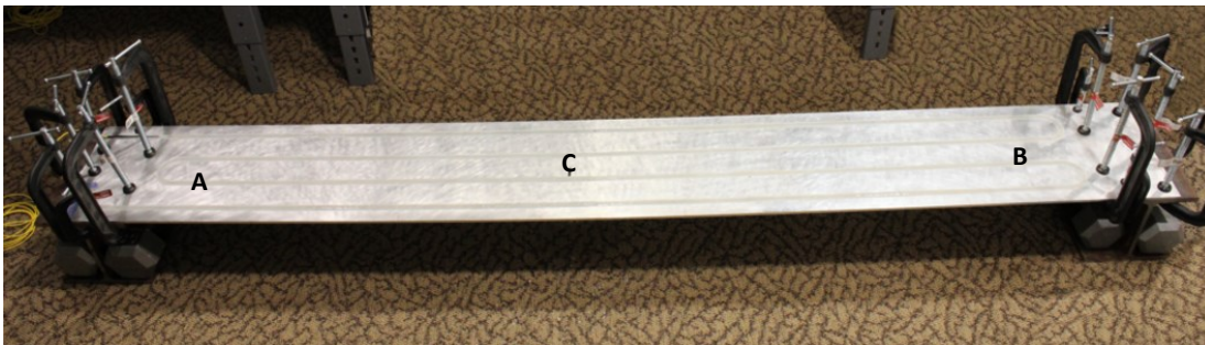
Figure 1. The test article instrumented with fiber is shown above. The severity of the inflicted damage is an 8.3% reduction in the moment of inertia. The location of the damage is indicated by the letter “C.”
