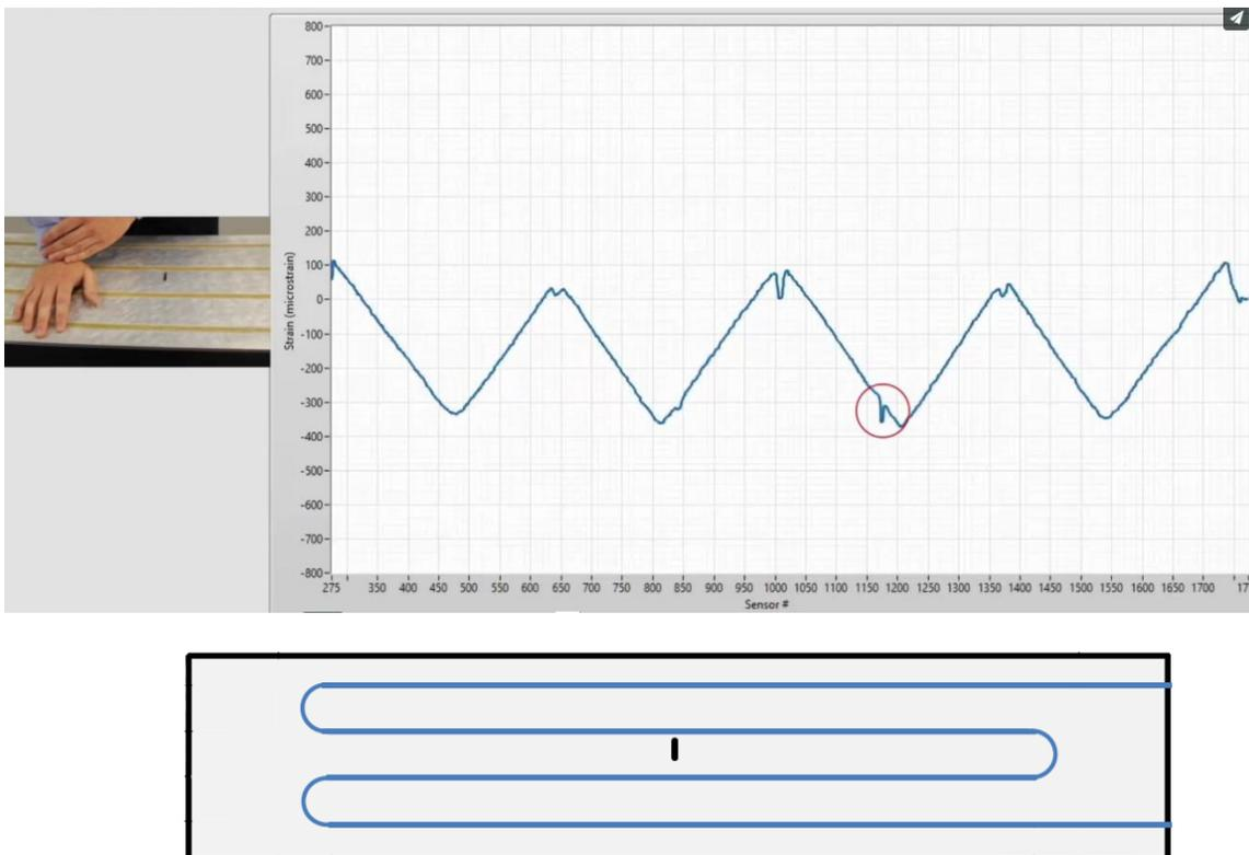
**Figure 2.** The top image shows the distributed strain data from a demonstration beam instrumented with approximately 10 m of fiber. The spike inside the red circle corresponds to a strain concentration around a crack in the beam. The bottom image is a diagram, illustrating in blue, the sensing fiber layout on the beam.
